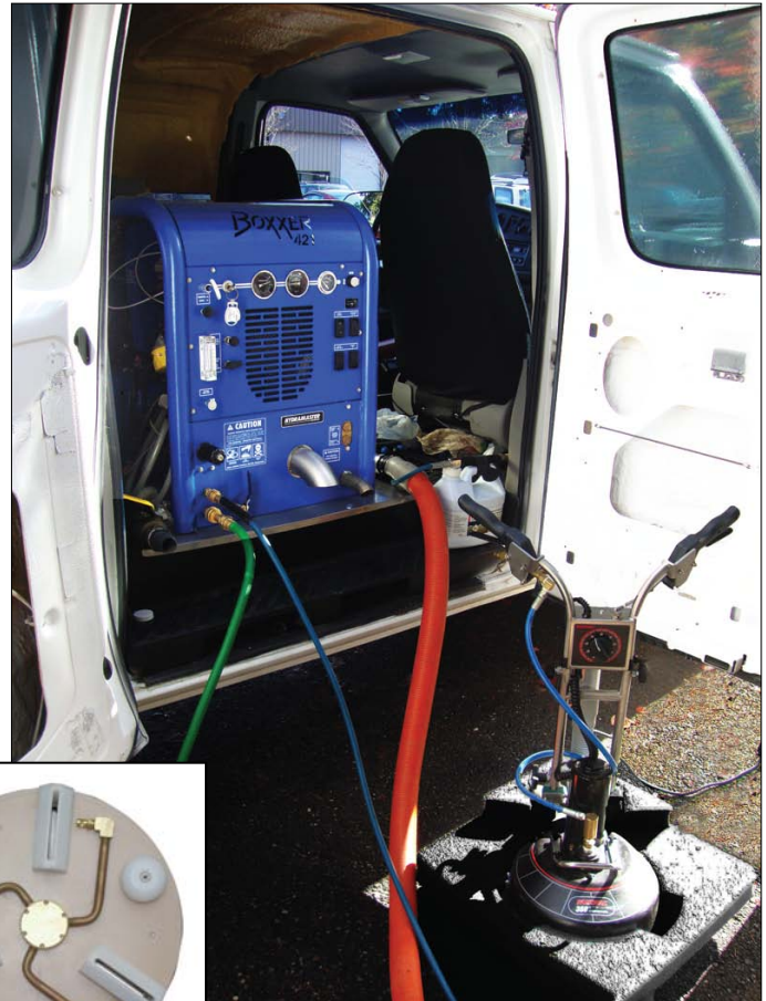
The Rotovac 360's oscillating head features three jets and three water intakes, and is powered by our top-of-the-line Boxxer truck mounted engine.
